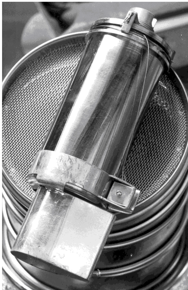
Figure 1: SESC used to collect soil sample 15013 from under Lunar Module. The wire was caught in the seal and the container was not under vacuum when opened. NASA S71-44784.
